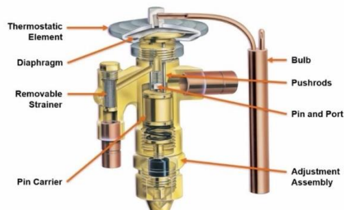
Fig 20: Thermostatic Expansion Valve (TXV) (left)
